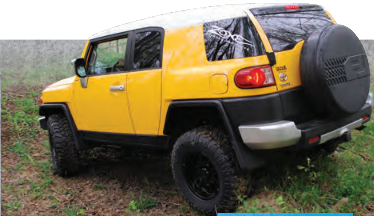
2.5" Lift Kit - 285/75r16 M/T MTZ - 16" M/T Sidebiter
